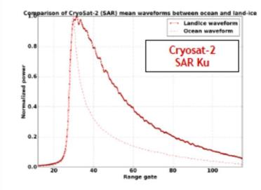
**SPICE** study (CLS) showed that volume echo (penetration) has minimal effect on the SAR Ku leading edge and so S3 SAR Ku tracks close to the surface.
